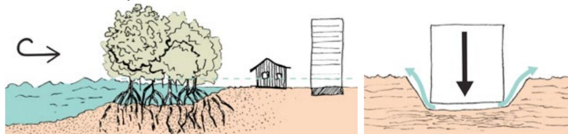
THE MANGROVE PROTECTS FROM WIND, COASTAL FLOODING AND EROSION. IT ACTS AS A WAVE/WIND CUTTER
